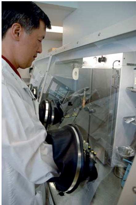
Working in an anaerobic glove box
